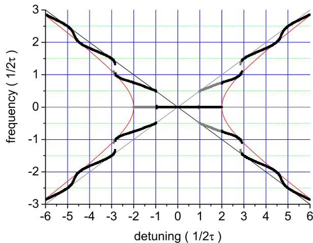
FIG. 1: Detuning scenario of the symmetrically detuned phase oscillators. Thick black: frequencies of both oscillators for increasing detuning. Thick grey: same for decreasing detuning. Thin lines: no coupling (grey) and no delay (red).
