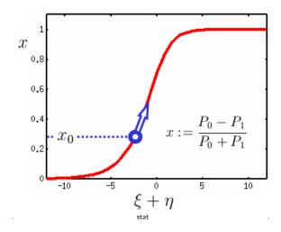
This general solution is shown in the Figure. It increases monotonically with normalized coordinate  $\xi$ . The only influence of the initial power ratio parameter  $x_0=x(z=0)$  is the starting point on this curve.
