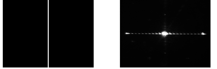
Figure 15: Input image of a slit with width b = 11 pixels (left) and its Fourier transform (right)
