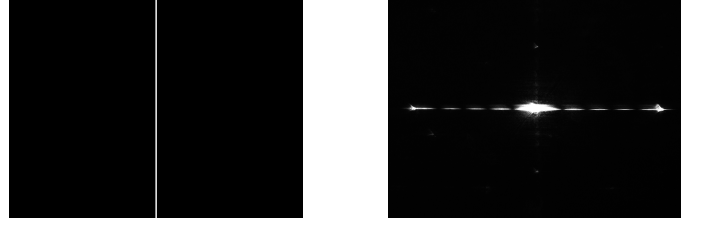
Figure 14: Input image of a slit with width b = 5 pixels (left) and its Fourier transform (right)
